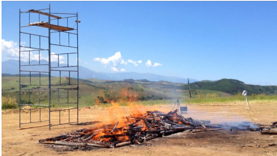
Small experimental fire implemented for the validation of same-day Landsat-8 and Suomi-NPP/VIIRS fire detection data in Brazil, Jan/2015. Tower-mounted radiometers provided 1Hz fire radiant flux data coincident with satellite overpasses.
