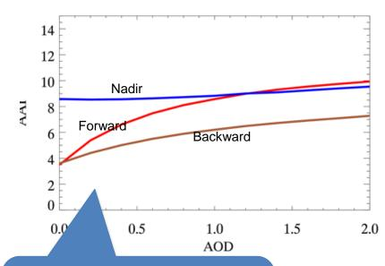
Theoretical calculations of AAI for three scenes corresponding to nadir, forward, backward scattering geometries
