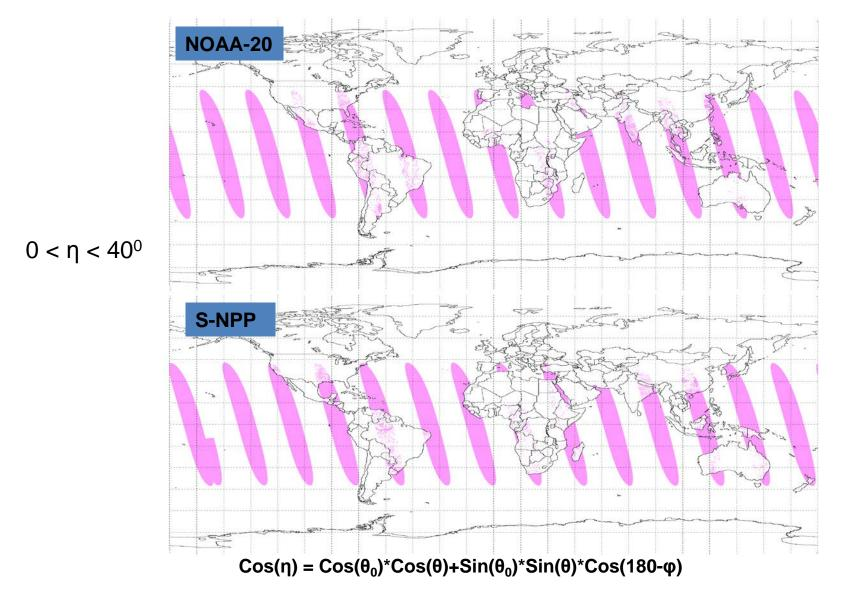
$\eta$  is the sunglint angle;  $\theta_0$  is the solar zenith angle  $\theta$  is the satellite zenith angle;  $\phi$  is the relative azimuth angle
