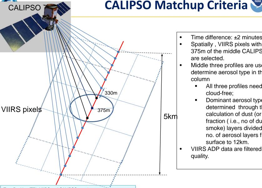
True Positive (TP): VIIRS and CALIPSO say dust True Negative(TN): VIIRS and CALIPSO say no dust False Negative(FN): VIIRS says no dust but CALIPSO says dust False Positive(FP): VIIRS says dust when CALIPSO says no dust
