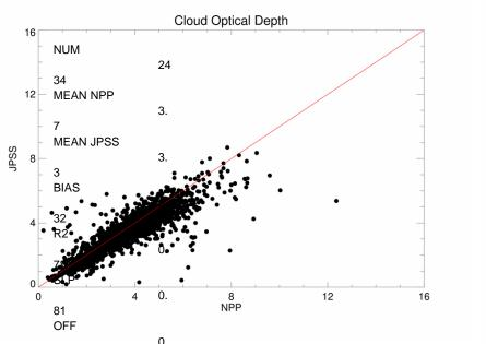
COD has a fair amount of expected scatter due to sampling differences. The bias is likely due to calibration for one or both of the instruments.
