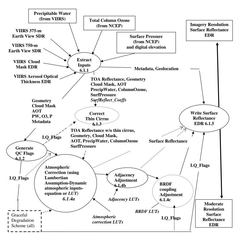
Figure 1. Surface Reflectance EDR processing architecture.
