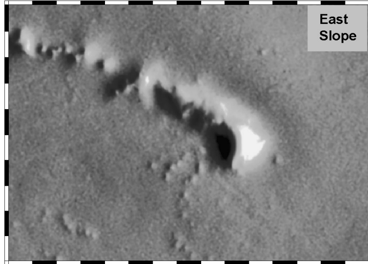
Figure 5. East component of sea surface slope \eta(\mathbf{x}) derived from Geosat and ERS altimeter profiles. Note this component is rather noisy because the altimeter tracks (Figure 3) run mainly in a N-S direction.
