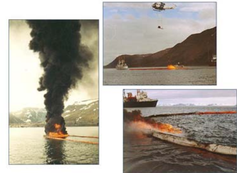
Testing of in-situ burning (igniters and booms) on Svalbard
