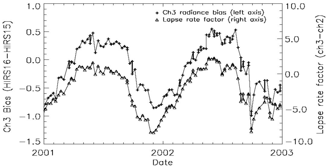
**Figure 2: Intersatellite radiance biases between HIRS on NOAA-15 and -16 show excellent agreement with uncertainties below the combined instrument noise. It also shows that seasonal variations in the bias are highly correlated with the lapse rate, indicating small spectral response differences between satellites.**
