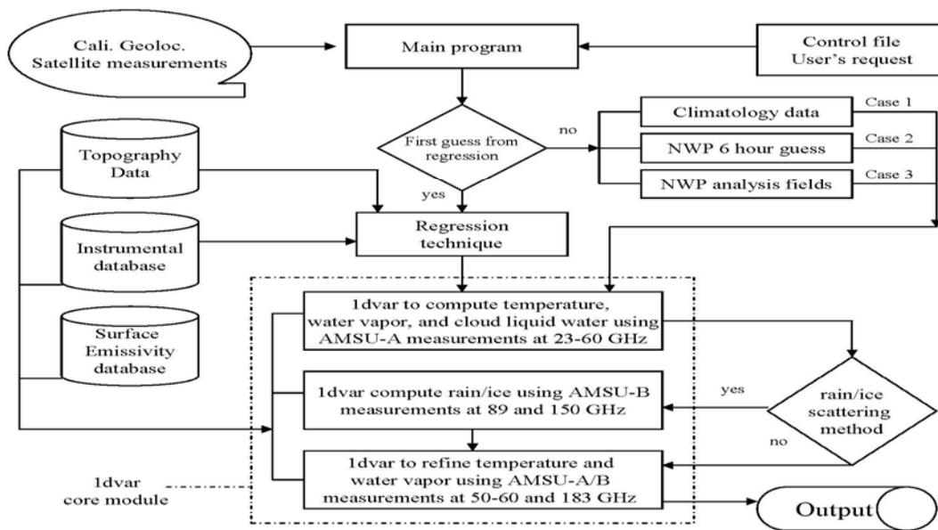
Figure 3: Flowchart of microwave integrated retrieval (MIR) system developed for future NPOESS era sensors such as ATMS and CMIS. The core module describes the retrieval procedures
