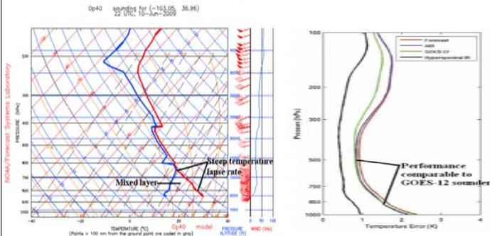
Figure 1. Prototypical "Inverted V" sounding profile, derived from Rapid Update Cycle (RUC) model analysis data at Kenton, Oklahoma at 2200 UTC 10 June 2009 (left), and temperature error curves for NWP forecast, ABI, GOES-12, and Hyperspectral IR soundings (courtesy Schmit et al. (2008), right).
