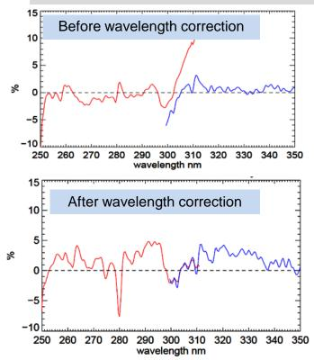
Wavelength dependent accuracy in cross-track scan direction exceed our expectation but can be corrected. The figure shows relative difference between measured and calculated NR
