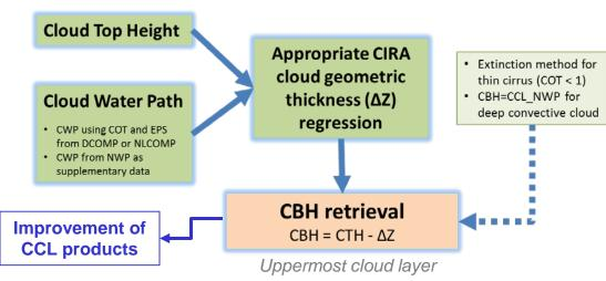
A new statistical CBH algorithm constrained by Cloud Top Height (CTH) & Cloud Water Path (CWP) using A-Train satellite data (described in Noh et al. 2017)
