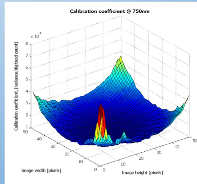
Examples of calibration coefficients for 50x50pixels. Done for all 138 bands
