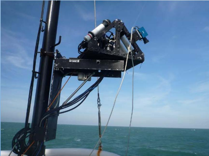
CCNY HyperSAS-POL (6 sensors) in front of the ship. Made at the stations and underway measurements with continuous adjustment of its platform for Sun glint minimization. Shown together with full Stokes green band camera.
