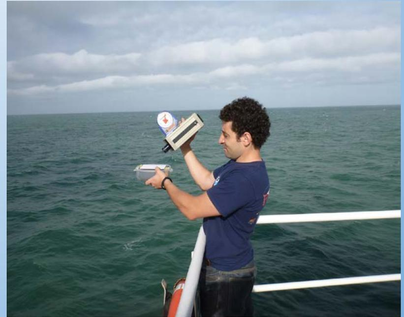
GER handheld spectroradiometer for manual operation
