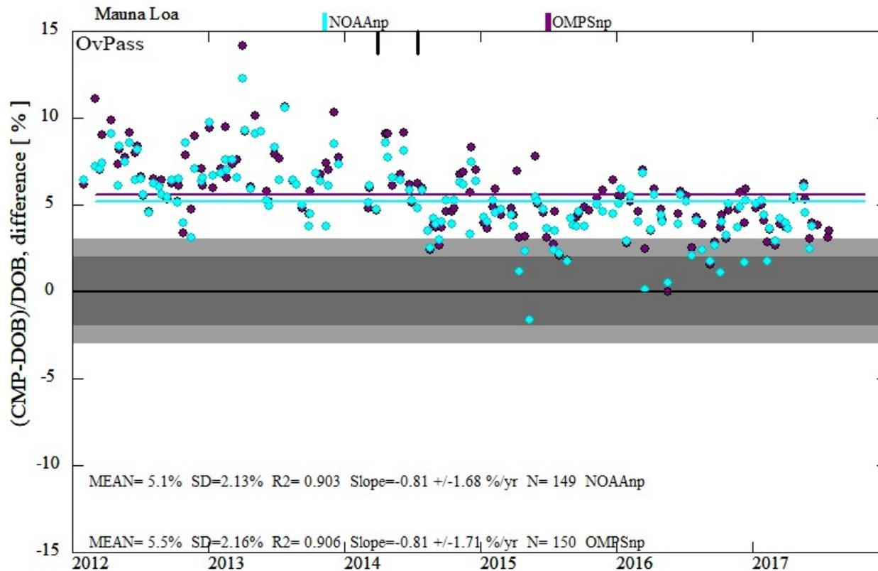
Apparent drift or step change in 2014, determined to be Dobson processing issue, ongoing work to correct for change in Q-table temperature sensitivity
