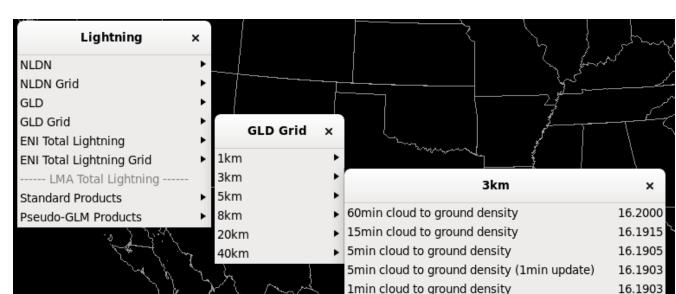
AWIPS operational lightning product menu (NLDN-Vaisala National Lightning Detection Network), GLD360 – Global Lightning Data from Vaisala, and ENI- Earth Networks Total Lightning. Pseudo-GLM is a GLD360 gridded product resampled to the 8 km x 8 km resolution of the GLM (in preparation for GLM data).
