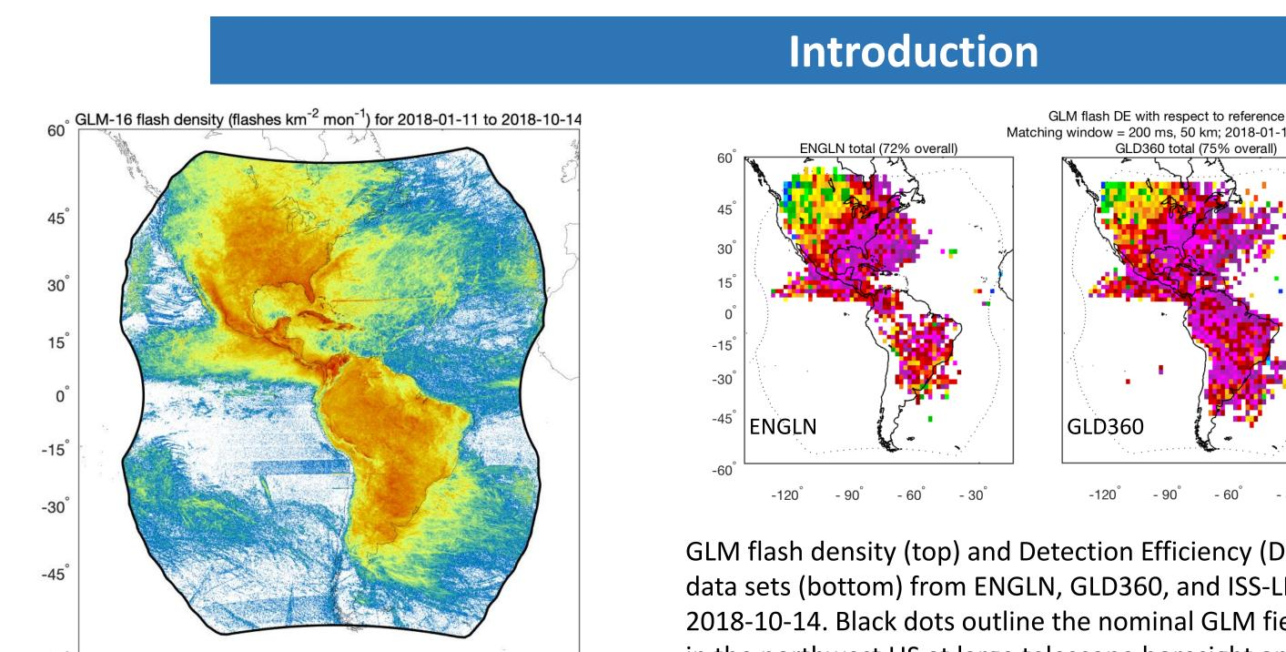
GLM flash density (top) and Detection Efficiency (DE) comparison with three reference data sets (bottom) from ENGLN, GLD360, and ISS-LIS for the period 2018-01-11 to 2018-10-14. Black dots outline the nominal GLM field of view. We find reduced GLM DE in the northwest US at large telescope boresight angle from both GOES-16/17. The ISS-LIS, having a nadir view and higher spatial resolution at nadir, detects lightning not as well observed by GLM.
