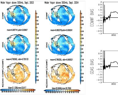
ECMWF computed radiances in water vapor band is 1.5 K closer agreement with AIRS than NCEP
