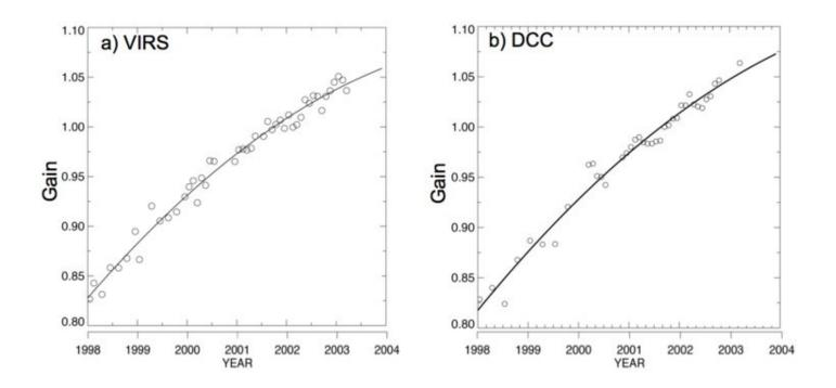
Monitoring of the GOES-8 visible (0.63µm) channel using the DCC and LEO/GEO inter-calibration methods.
