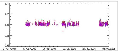
Time series of the ratio of the ESA MERIS to NASA MODIS 0.665 micron visible channel reflectance from observations at 19 desert sites in North Africa and Saudi Arabia.
