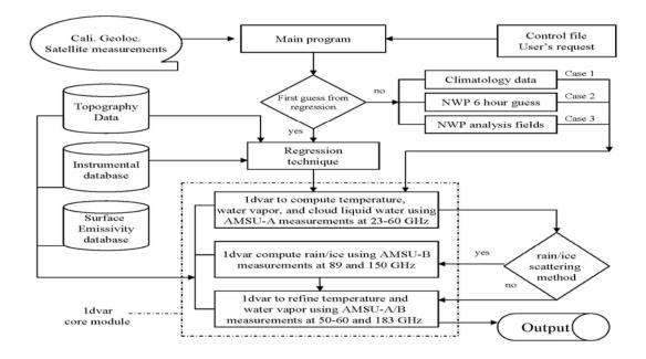
Figure 3: Flowchart of microwave integrated retrieval (MIR) system developed for future NPOESS era sensors such as ATMS and CMIS. The core module describes the retrieval procedures
